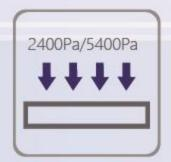
Certified to withstand 2400 Pa of wind load and 5400 Pa of snow load
